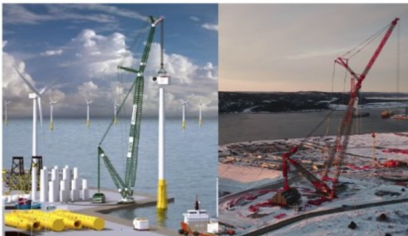
Huisman and BMS crane (left), Mammoet SK350 crane (right).
